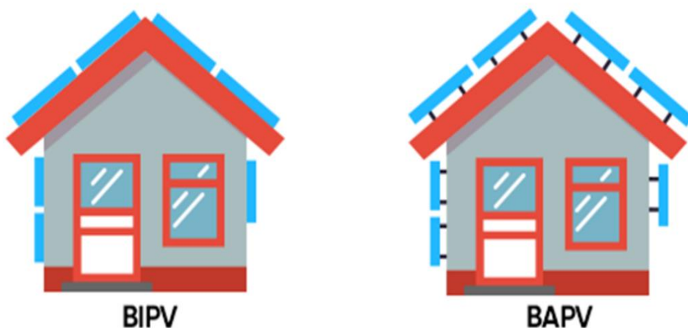
Figure 2.12 The variations between BAPV and BIPV.
