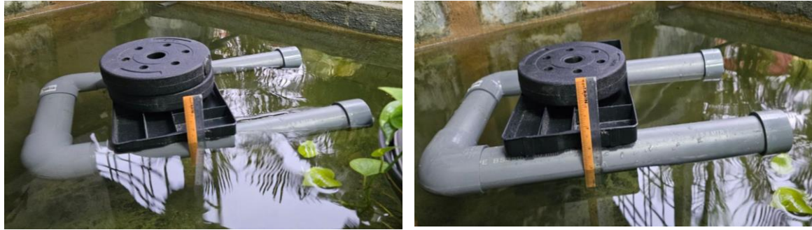
Figure 3.6 : Floating test with Load
