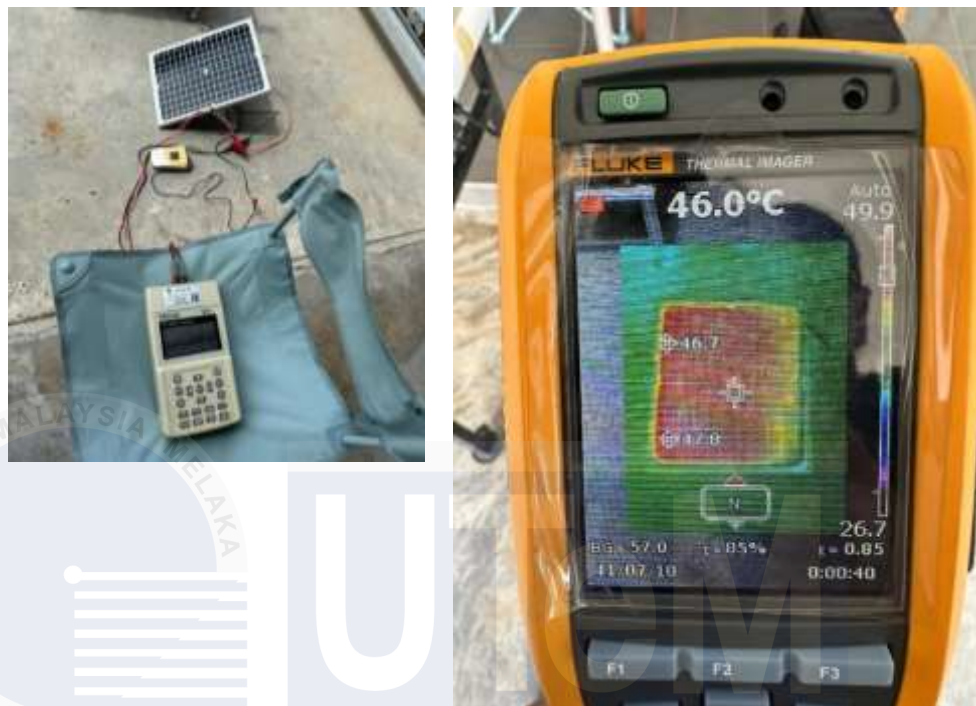
Figure 3.15 Solar panel testing setup
