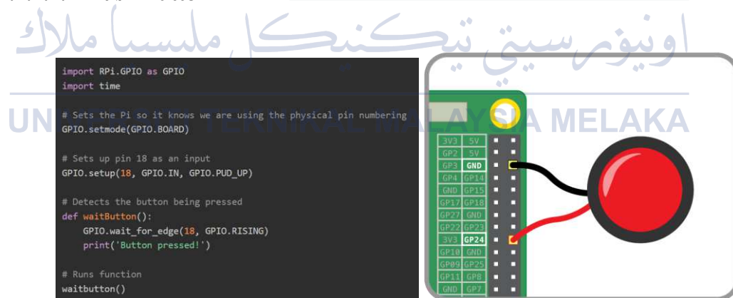
Figure 3.6 Basic Coding and Circuit for Push Button
