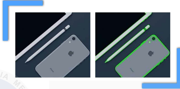
Figure 2.6 Contour Detection Technique Detect Phone and pencils
