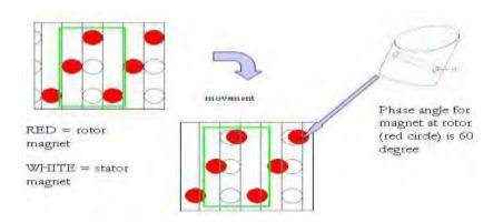
Figure 2.1: The magnets on the rotor being off-set to produce rotation
