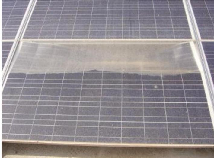
Figure 2.15 Delamination defect on a photovoltaic panel.
