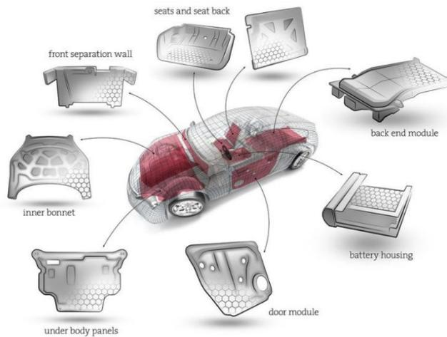
**Figure 2.1** Possible applications Organosandwich (Pflug & Schlimper, n.d.)
