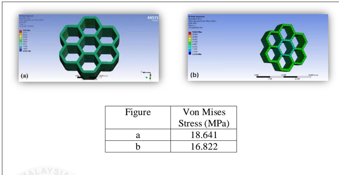
**Figure 3.6** (a) desired von mises stress and (Chandrashekhar, et al., 2020) (b) generated von mises stress, of honeycomb structure
