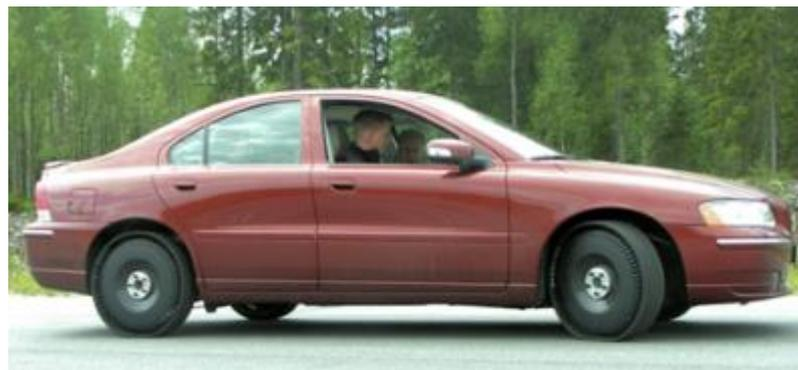
**Figure 2.3** The Composite Wheels mounted on a Volvo car for various tests (Sandberg, 2020)
