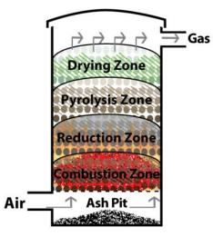
Figure 2.1: Four Zone Process in Updarft-Gasifier
