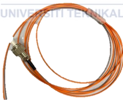
Figure 3.10: Pigtail probe for Single Mode and Multimode
