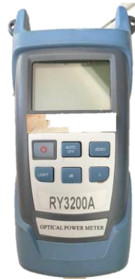
Figure 3.11: RUIYAN RY3200A Optical Power Meter
