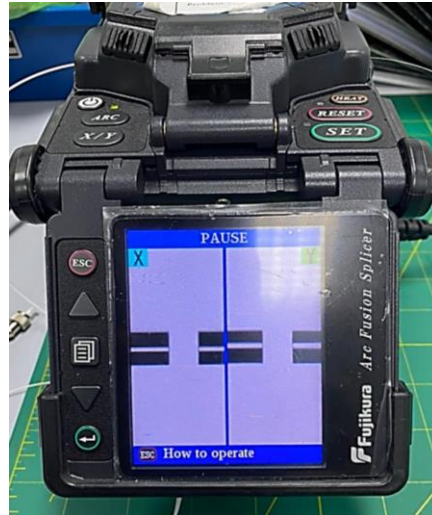
Figure 3.3: Procedure of Setting up the Normal Fusion Splicing using Fujikura FSM 18-R
