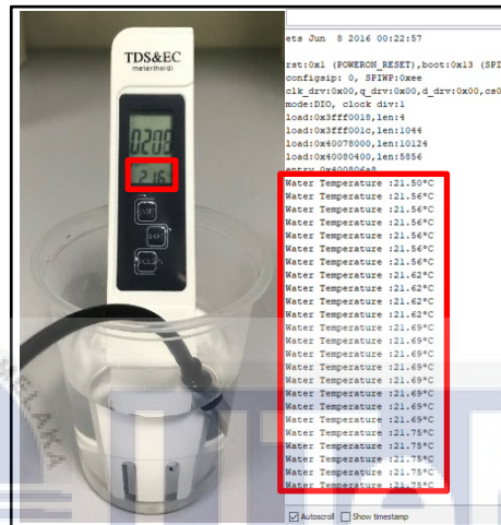
Figure 4.5: Result Between Water Temperature Sensor and Water Temperature Device.
