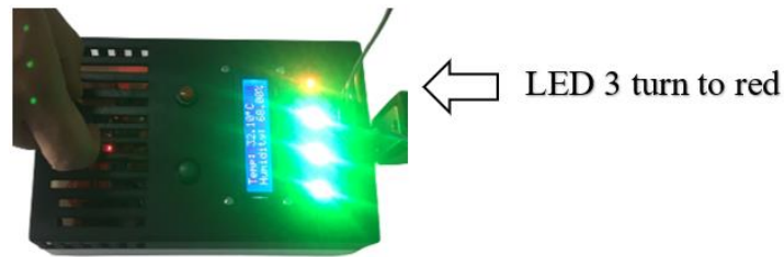
Figure 4. 10 Output when combustion gas detected
