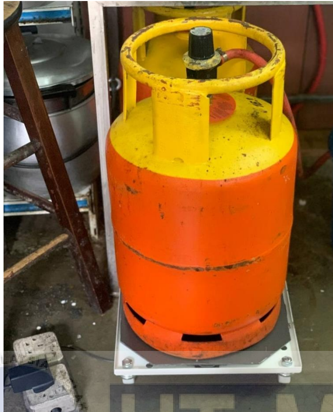
Figure 4.5: Testing the LPG Cylinder Weight For 23mins (In Use)
