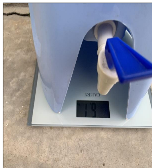
Figure 4.6: Testing Load Sensor with Water Dispenser
