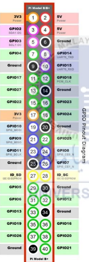
Figure 3.6: GPIO Pinout Raspberry Pi 3 Model B
