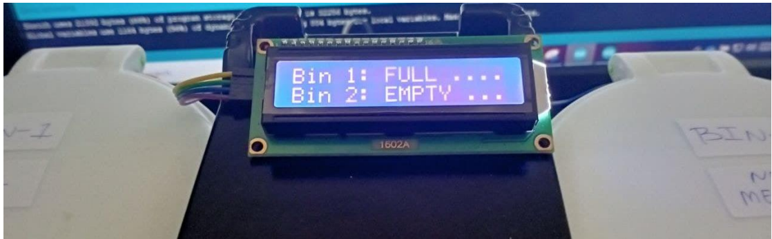
Figure 4.5: LCD display the current level of waste for both Bin 1 and Bin 2.
