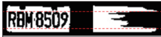
Figure 2.27: Eliminating the upper and lower borders by horizontal projection [4]
