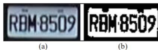
Figure 2.26: (a) An example of a detected vehicle license plate, (b) a binarized plate [4]
