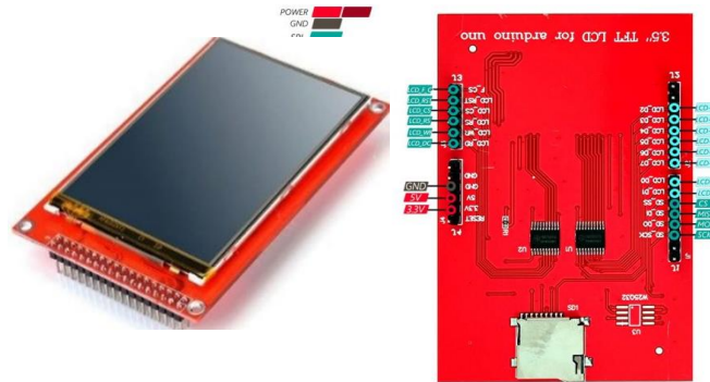
Figure 3. 15: 3.5 inch TFT display output pin.
