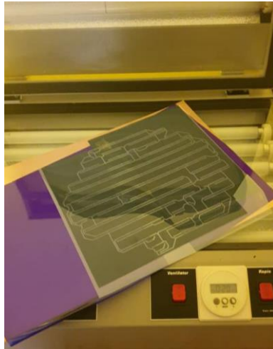
Figure 3.13: PCB Ultra Violet Rays in the UV Chamber
