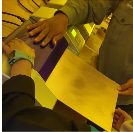
Figure 3.11: Laminating photo-lith film
