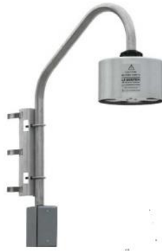
Figure 3.1: Electric field mill (EFM) sensor [41].
