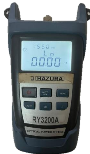
Figure 3.16: Optical Power Meter
