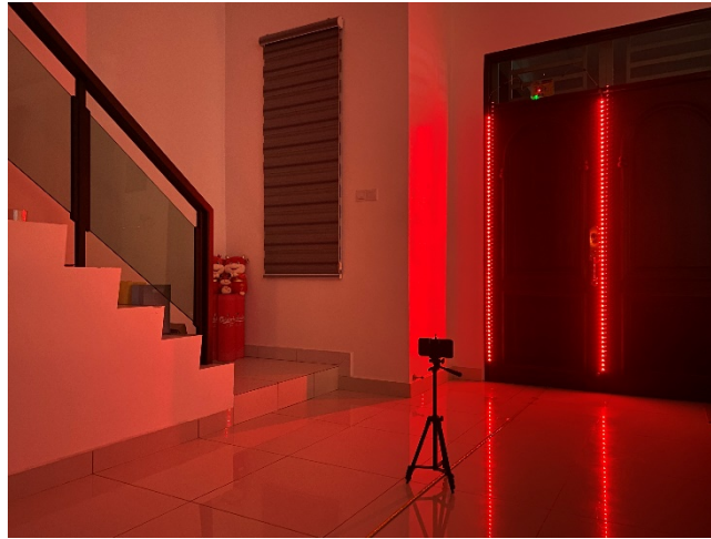
Figure 3.21 (a): Luminosity measurement of red LEDs
