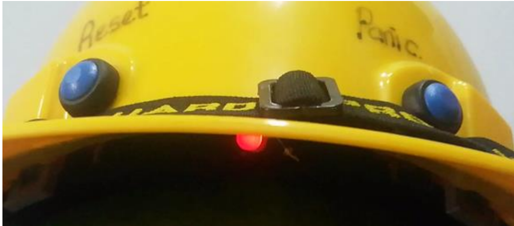
Figure 4.17: Red LED on the helmet to indicate the created alarm at the dashboard
