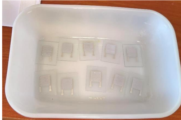
Figure 4.4.4.3: Titanium paste added on second layer of glass substrate
