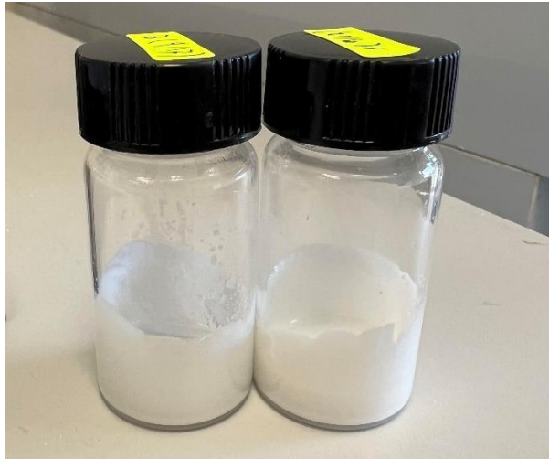
Figure 4.4.2.1: Paste obtained from the mixture of binder and titanium (IV) oxide nano powder
