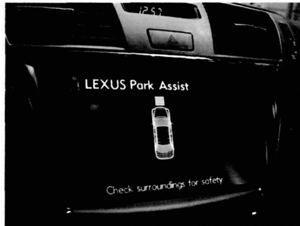
Figure 2.1 : Lexus LS 460L control panel in park assist mode [1]
