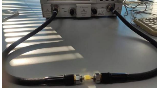
Figure 4.7.1.1: Split ring resonator based sensor test MUT by network analyzer
