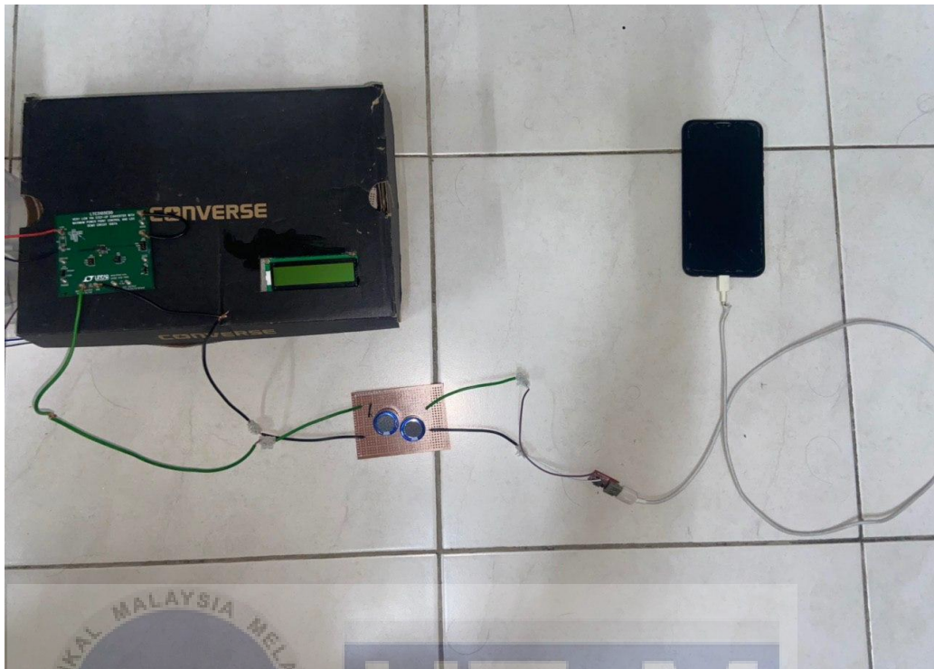
Figure 3.6 The second part of prototype which the output of supercapacitor goes into the 5V usb converter and the output will go into the mobile phone
