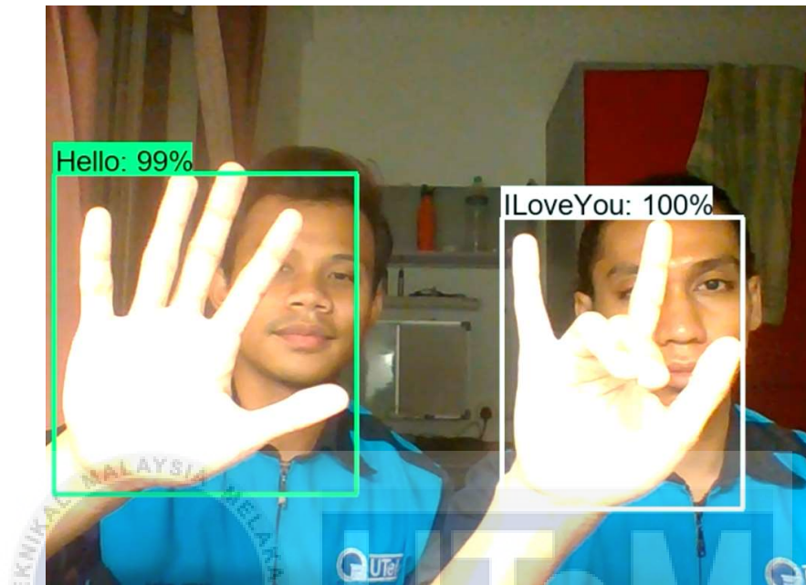
Figure 4.19: Sign gesture with two people in real time for Hello 99% and I Love You 100%
