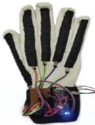
Figure 2.10: Prototype of the designed glove uses low-cost hardware.
