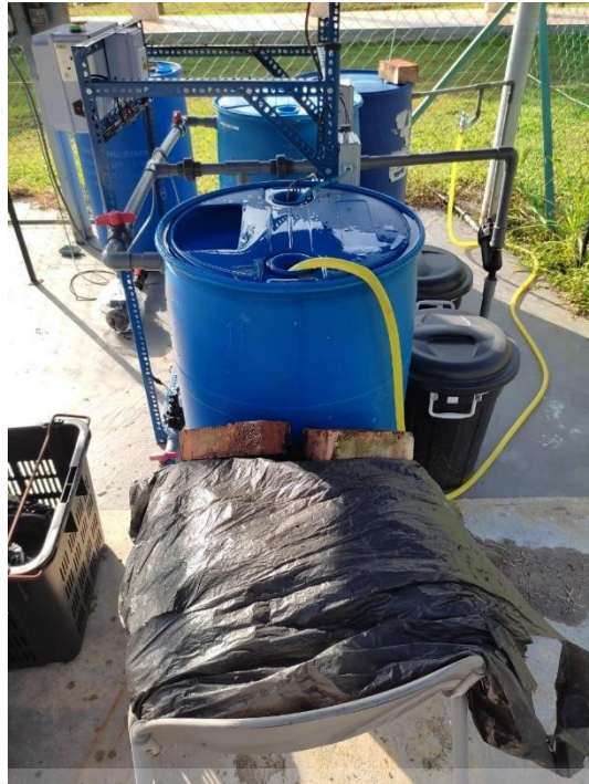
Figure 9 : CRIM IOT fertigation system
