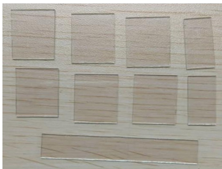
Figure 11 ITO Coated Glass that conduct electricity used as electrode and holder for this project
