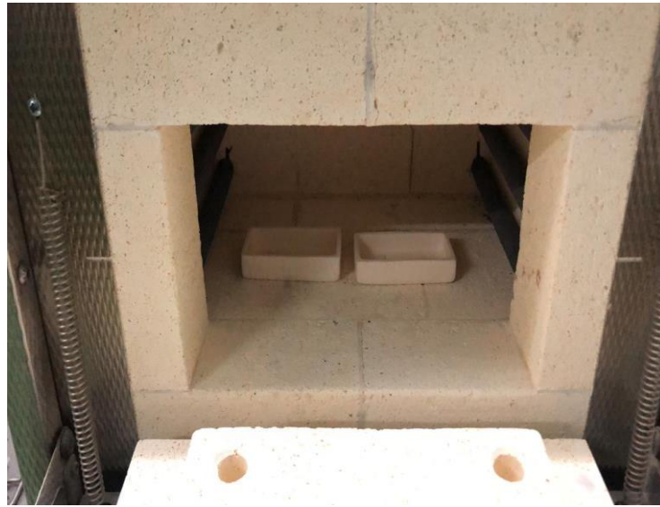
Figure 15 Furnace for annealing 250celsius for 5hours
