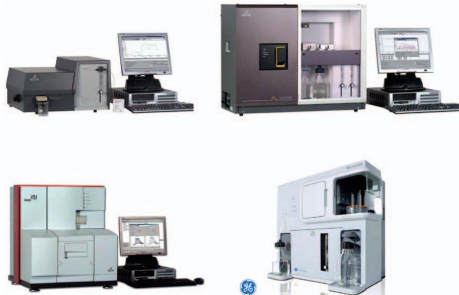
**Figure 2.4: In the SPR product line of Biacore: X, 3000, S51, and X100, respectively.**
