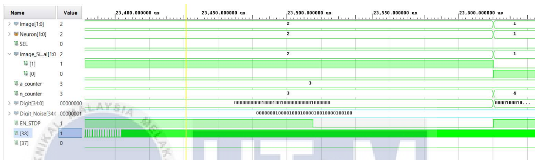
Figure 4.12: Neuron 37 spikes to classify record number 103 correctly as normal.
