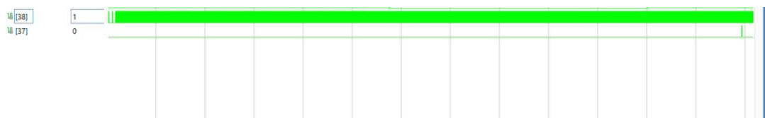
Figure 4.14: The incorrect output neuron randomly spikes while the correct output neuron is spiking.
