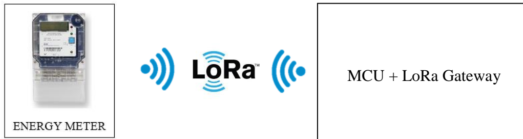
Figure 2.5: Smart Energy Meter system using LoRa network [11] [17].
