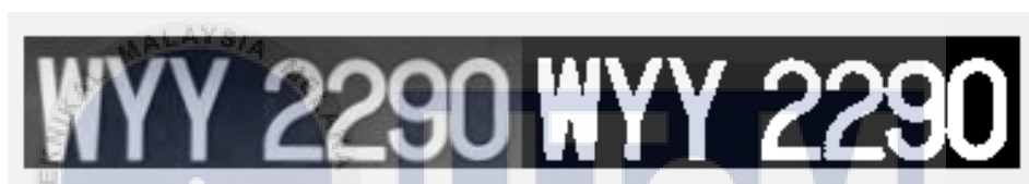
Figure 2.1: Greyscale Image (left) and Binary Image (Right)
