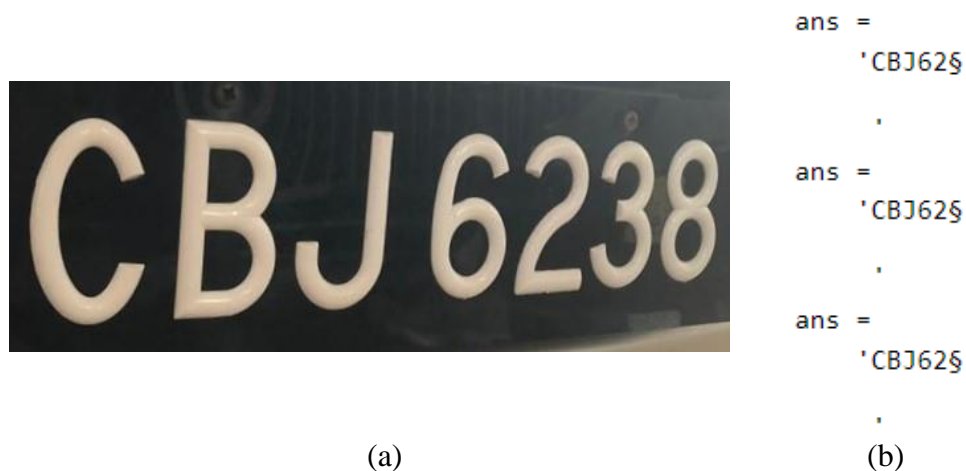
Figure 4.5: (a) Side Image of Car Plate (b) OCR Result
