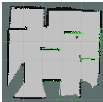
Figure 4.16: Environment map created for 50 seconds when speed is  $1.0\text{ms}^{-1}$ .
