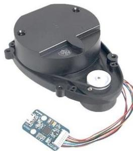
Figure 3.4: 360 Laser Distance Sensor LDS-01 (LIDAR).
