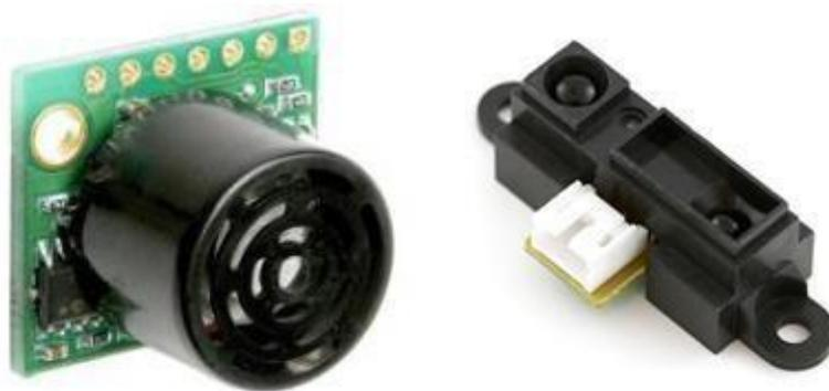
Figure 2.14: Ultrasonic and Infra-red Range Sensor.
