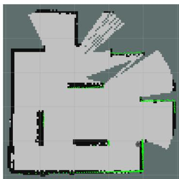
Figure 4.10: Environment map created for 40 seconds when speed is  $0.5\text{ms}^{-1}$ .
