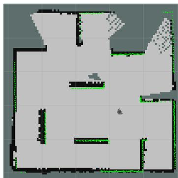
Figure 4.11: Environment map created for 50 seconds when speed is  $0.5\text{ms}^{-1}$ .
