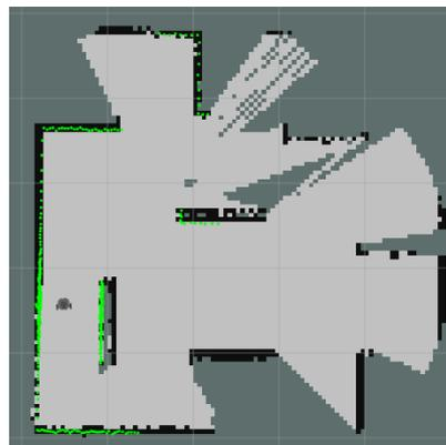
Figure 4.9: Environment map created for 30 seconds when speed is  $0.5\text{ms}^{-1}$ .
