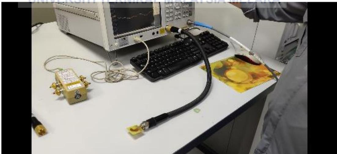
**Figure 3.54: Connections of antenna to VNA**
