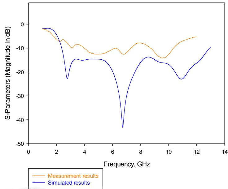
**Figure 4.5: Comparison return loss for simulation and measurement results for irregular patch antenna**
