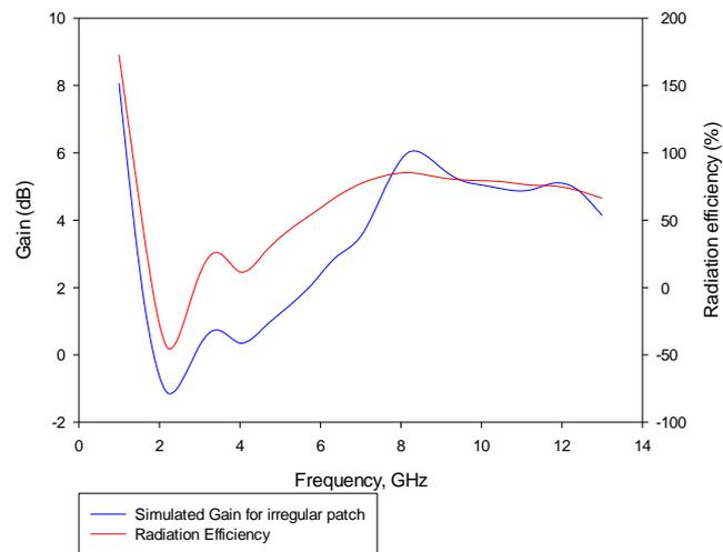
**Figure 4.10: Gain and Radiation Efficiency Curve for Irregular Patch Antenna**
