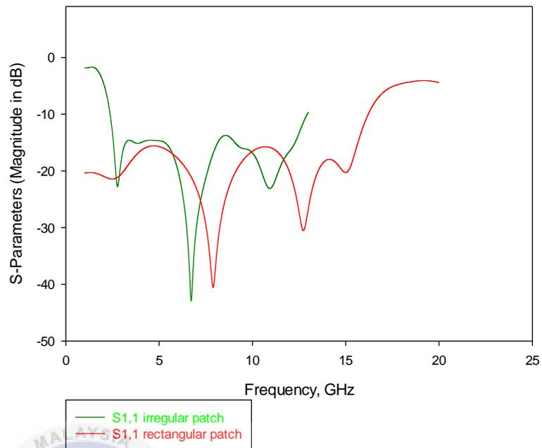
**Figure 4.3: Comparison of Return Loss Between Rectangular and Irregular Patch Antenna**
