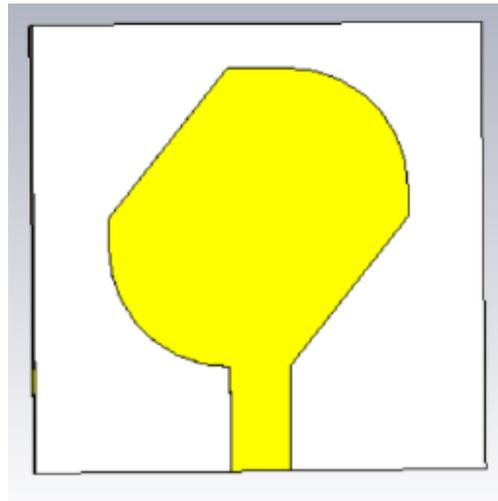
**Figure 3.41: Front View of the Leaf-shaped Patch Where Edges Have Been Cut**
