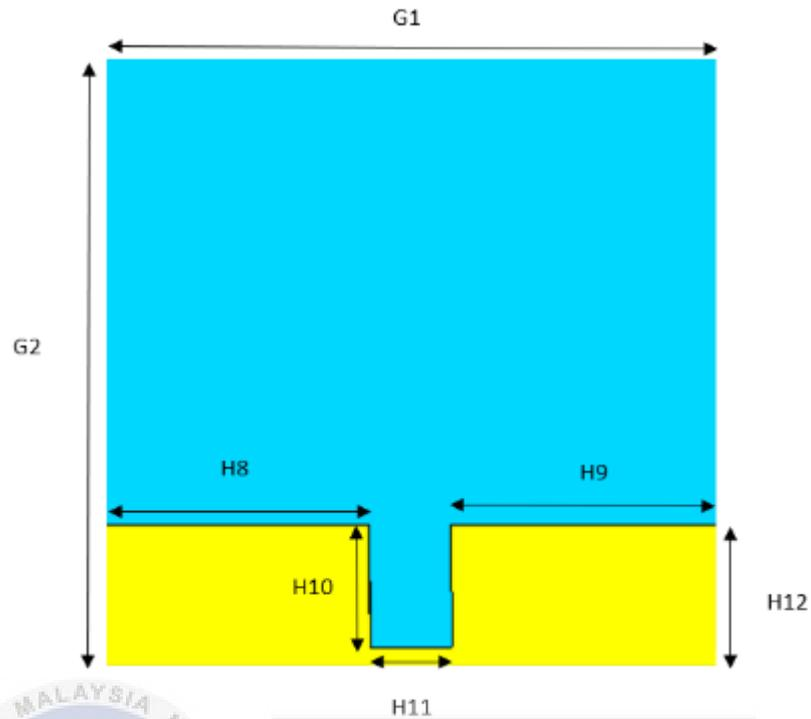
**Figure 3.4: Back View for the Irregular Patch**
