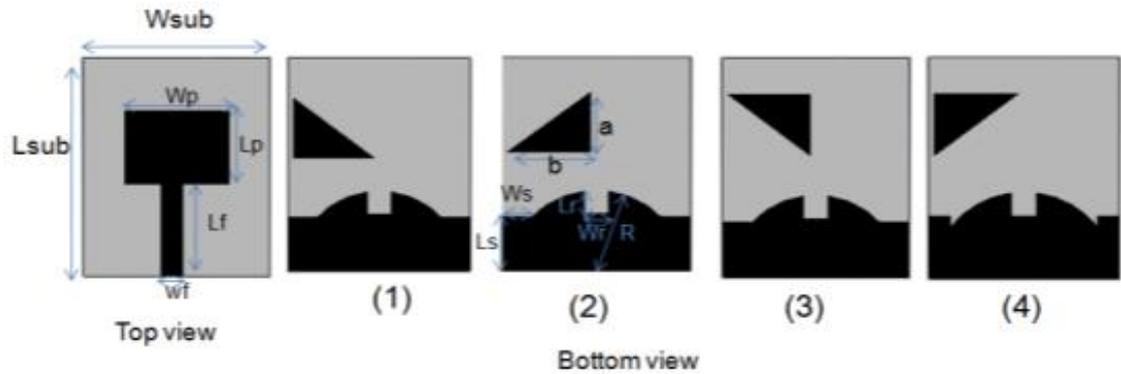
**Figure 2.13: Rectangular Radiating Plane with Different Positions of Additional Ground Plane**
