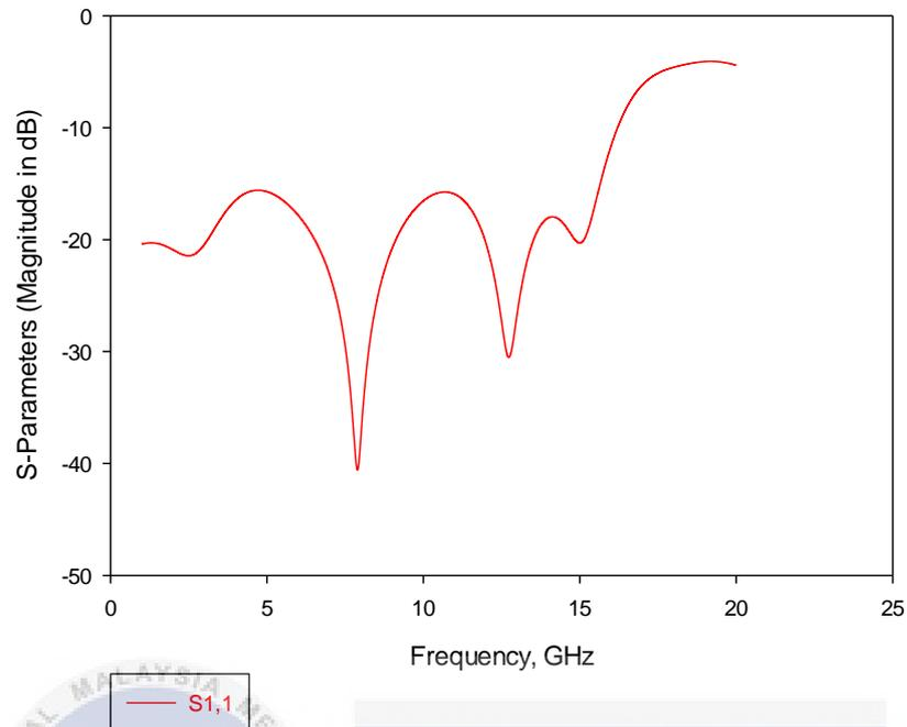
**Figure 4.1: Return Loss for Rectangular Patch Antenna**
