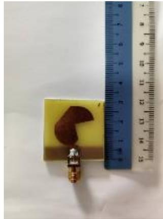
**Figure 3.52: Front view for irregular patch antenna**
