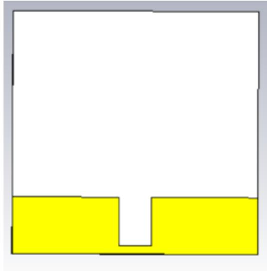
**Figure 3.44: Back View of the Ground That Has A Slot Has Been Etched on It**
