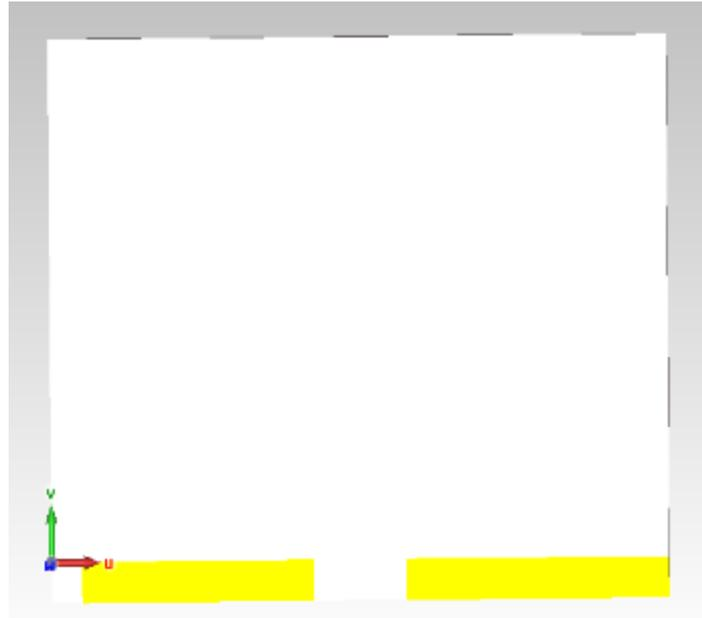
**Figure 3.28: Ground Plane Second Slot with the Size 1.1 mm x 1mm**
