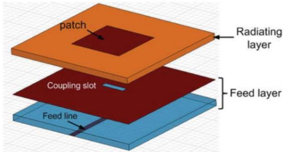
**Figure 2.2: Aperture Coupled Feed**
