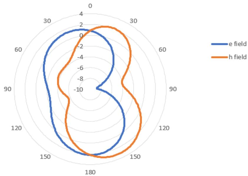
Figure 4.16: Simulation radiation pattern at 6.7 GHz
