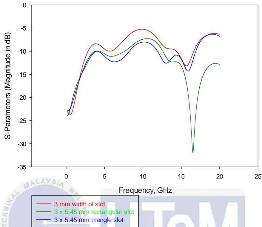
Figure 3.17: S-parameters for 3 mm x 5.45 mm Square and Triangle Slot
