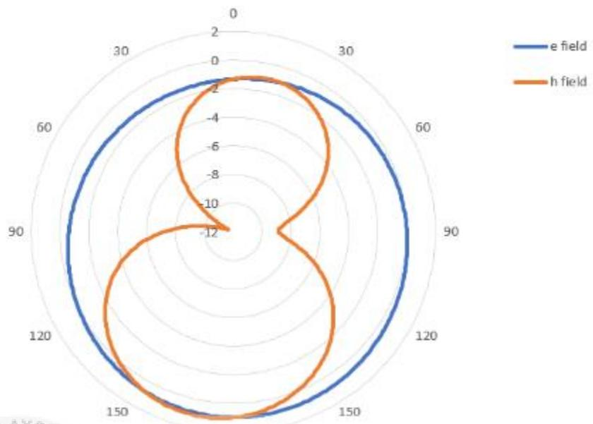
Figure 4.14: Simulation radiation pattern at 2.8 GHz
