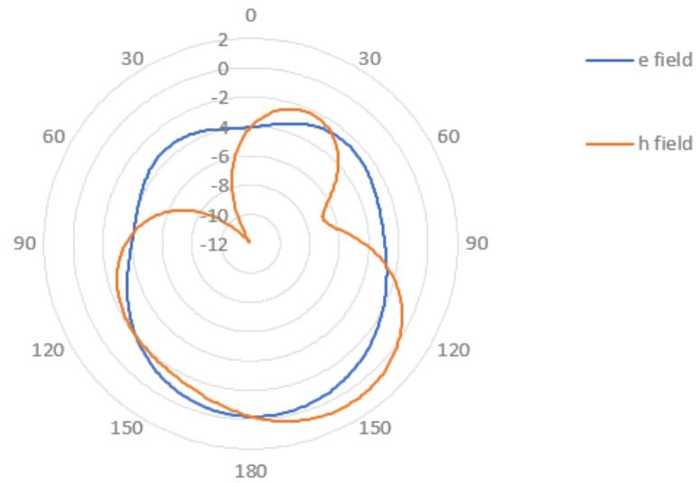
**Figure 4.12: Simulation radiation pattern at 7.9 GHz**
