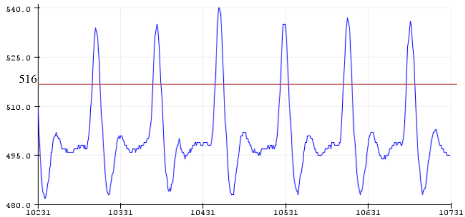
Figure 4.5 PPG signal from Arduino serial plotter
