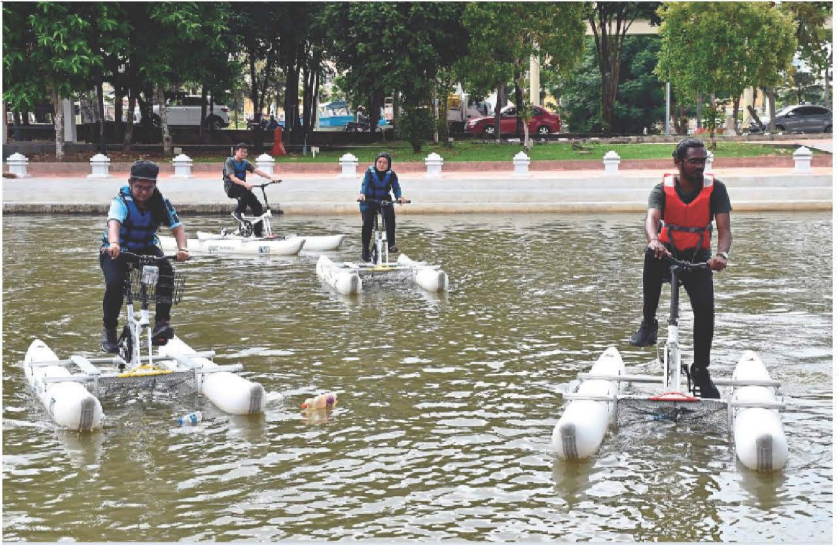
The water bikes developed by a group of UTeM lecturers and students feature a trash trap to clean up floating debris.
