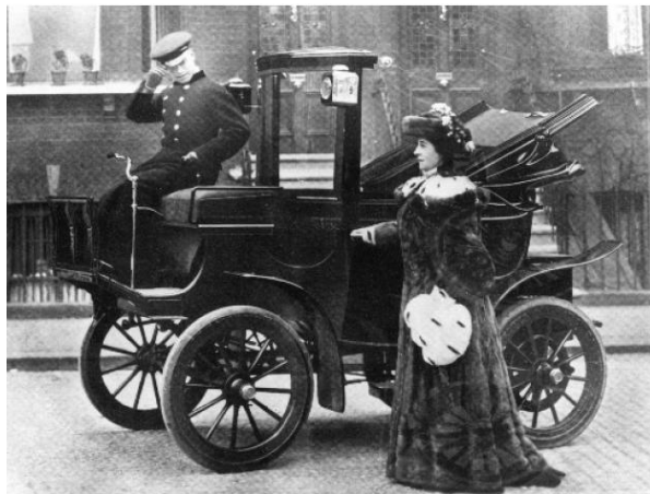
Figure 2.1 New York taxi cab in about 1901, a battery electric vehicle (Larminie and Lowry, 2003)
