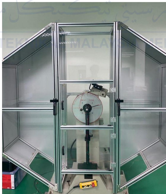
Figure 3.2 JBW-500 Computer Pendulum Impact Testing Machine
