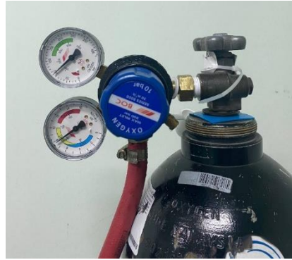
Figure 2.4 Type of gas used in SLM process (oxygen, O 2 )
