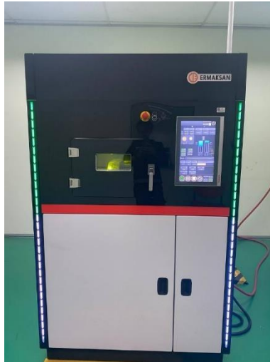
Figure 2.16 Ermaksan Enavivion 120 SLM 3D Metal Printer
