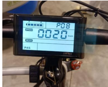
Figure 3-5: Setting Speed to 20 km/h
