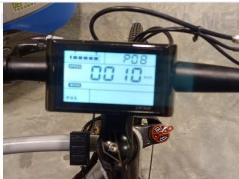
Figure 3-4: Setting Speed to 10 km/h
