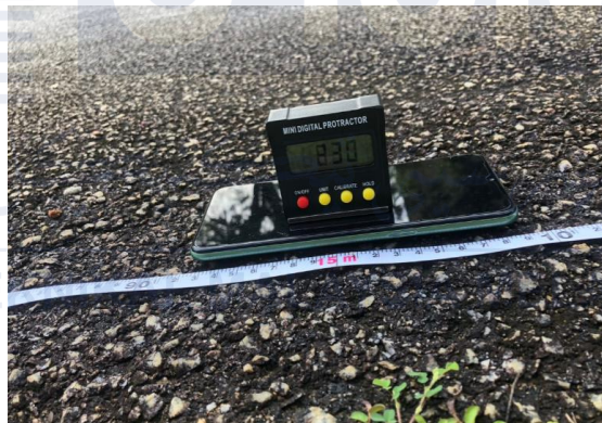
Figure 3-10: Measuring angle of Inclination using Digital Protactor
