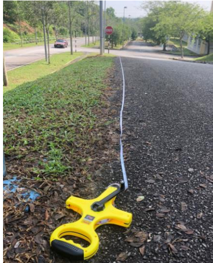
Figure 3-9: Measuring 30 meter using measure tape
