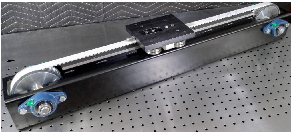
Figure 2.4: Timing Belt and Pulley
