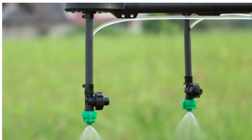
Figure 1.5: Fixed-Typed Pesticide Spraying System
