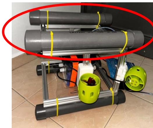
Figure 3-9: Upper PVC Pipe (Buoyancy Tank)
