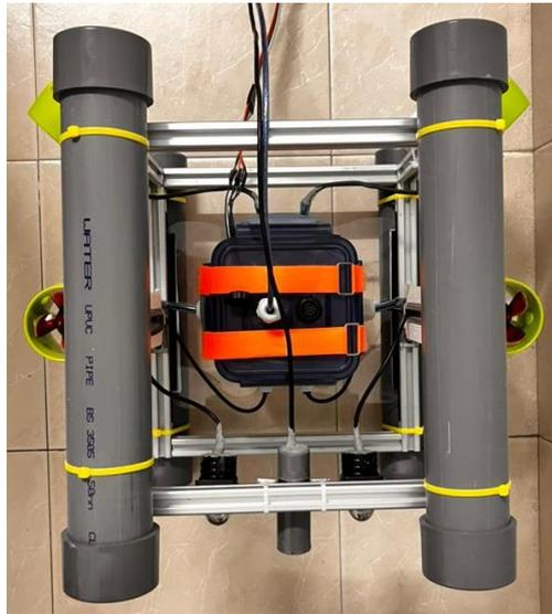
Figure 4-2: Top View of ROV Prototype
