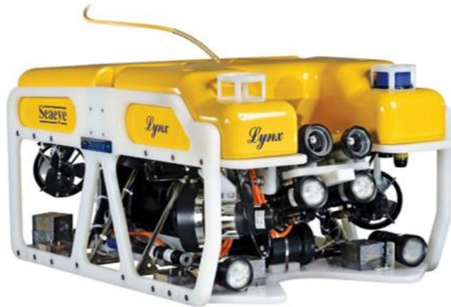
Figure 2-2: Example of Observation ROV[9]
