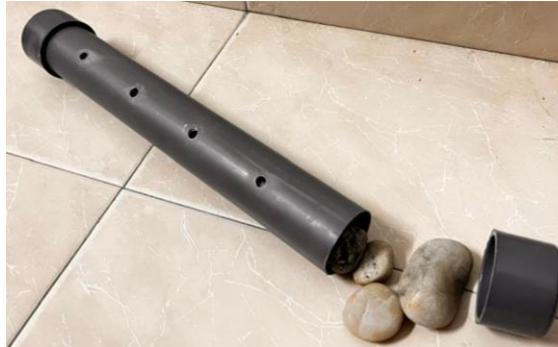
Figure 3-10: Bottom PVC Pipe (Ballast Tank)
