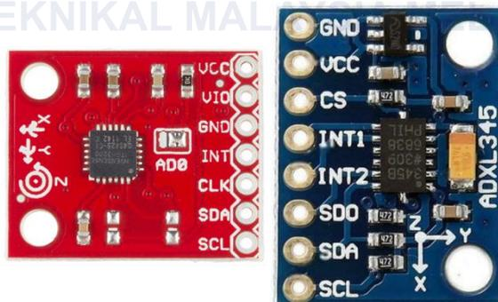
Figure 2-20: IMU Digital Combo Board – 6 degrees of freedom ITG3200/ADXL345 [52]
