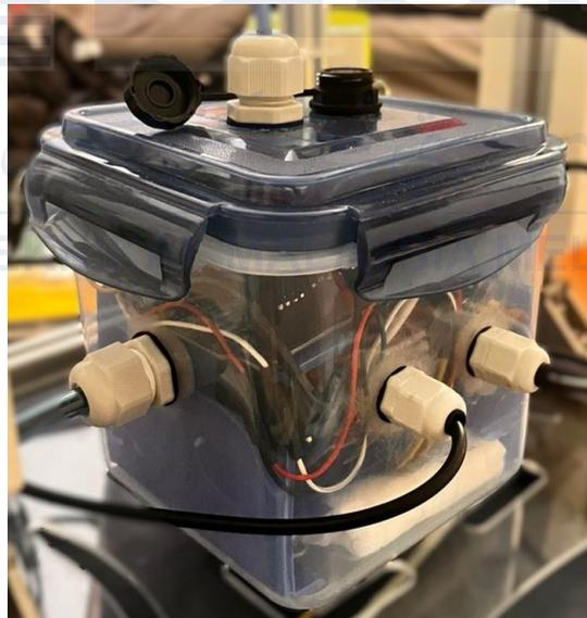
Figure 4-5: Leakproof Food Container (Pressure Hull)
