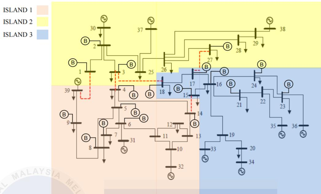
Figure 4.11: One-Line Diagram for Case Study 4 After Integrating BESS
