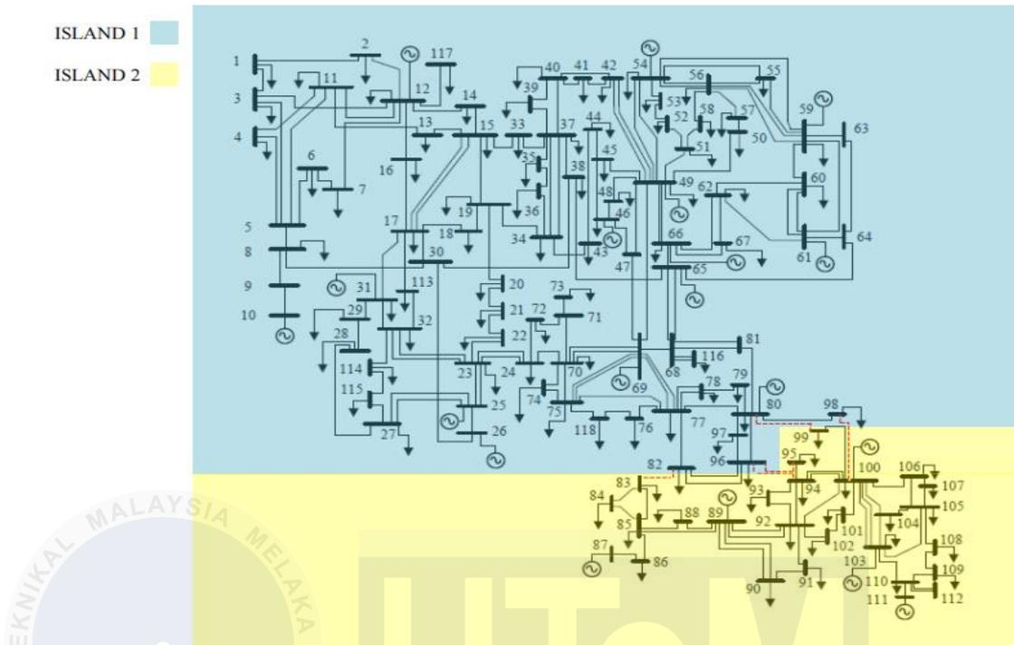
Figure 4.12: One-Line Diagram for Case Study 5 Before Integrating BESS
