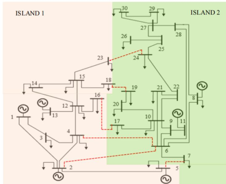
Figure 2.2: One line diagram for IEEE 30-bus system using MDEP
