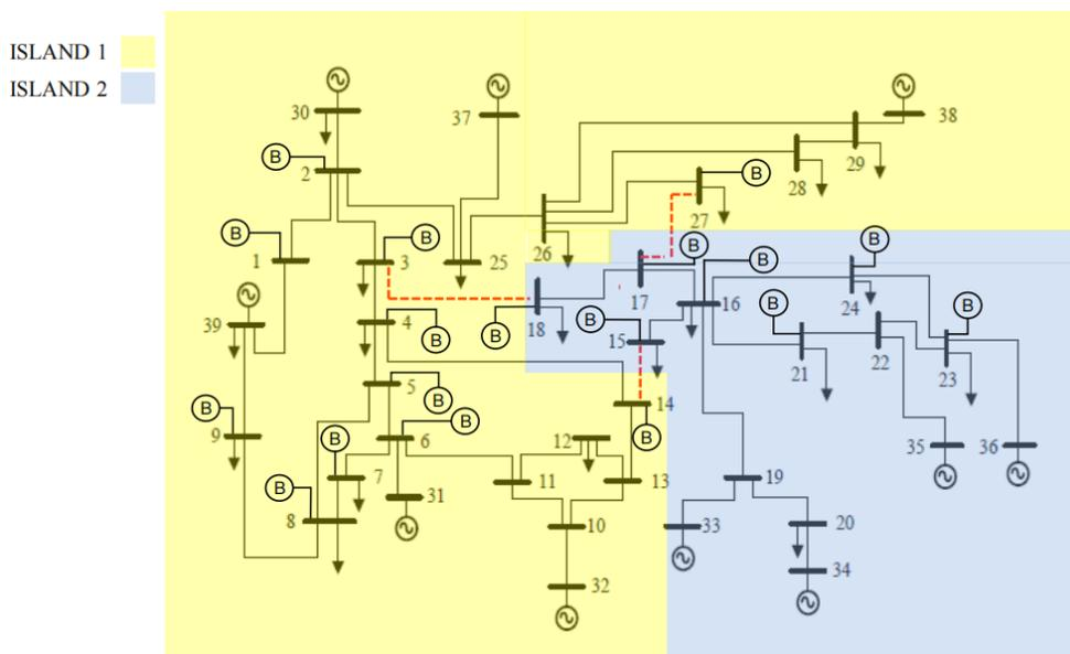
Figure 4.9: One-Line Diagram for Case Study 3 After Integrating BESS
