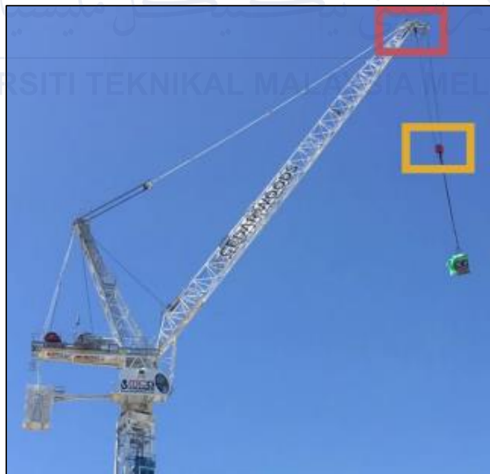
Figure 1-1: A tower crane equipped with a retractable hoist rope [1]
