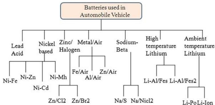
Figure 2.9 : Battery Used In Automobile Vehicle[3].
