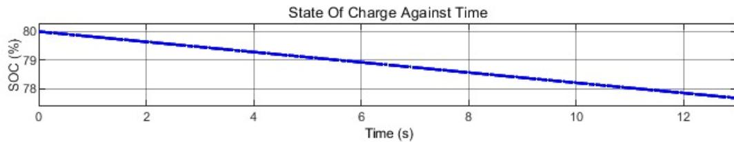
Figure 4.11 : SOC of battery for buck mode
