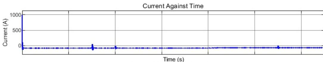
Figure 4.3 : Battery current for boost mode
