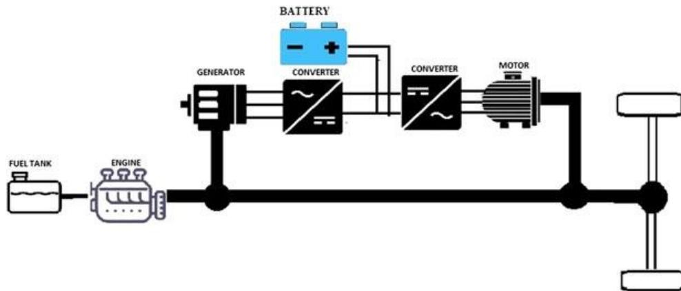
Figure 2.3 : Series-Parallel drive train structure[3].
