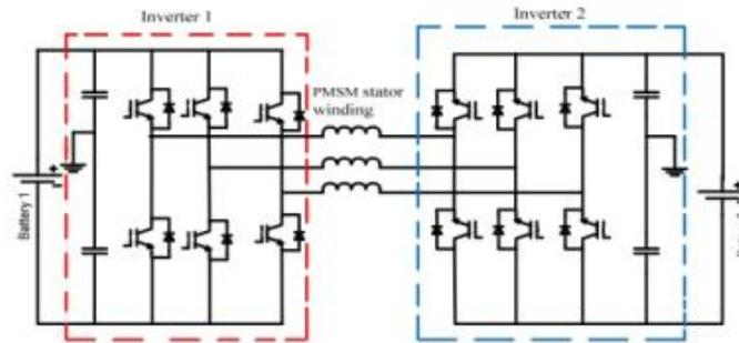
Figure 2.14 : Bidirectional converter with single and dual source [3]
