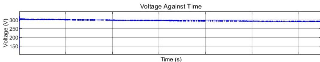
Figure 4.7 : Battery voltage for buck mode
