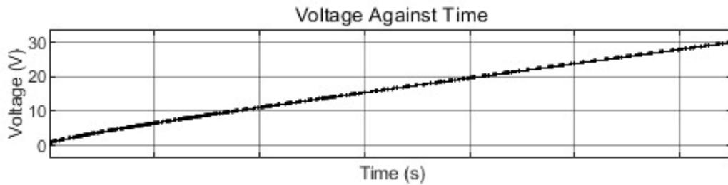
Figure 4.8 : Supercapacitor voltage for buck mode
