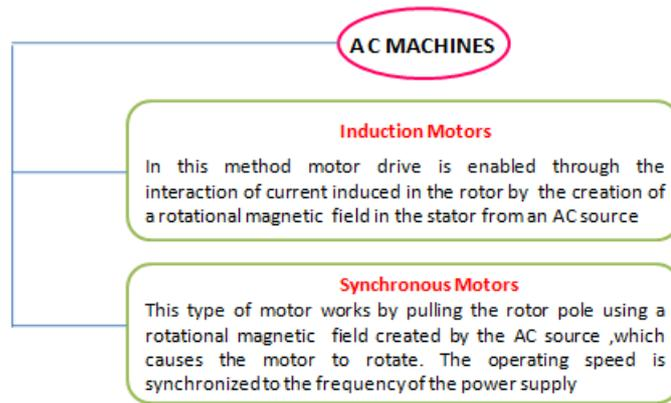
Figure 2.19 : Classification of AC Electrical motors[27].
