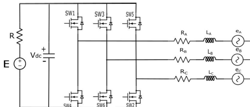
Figure 3.11 : Circuit diagram of BLDC Motor
