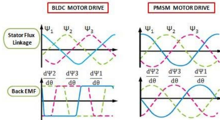
Figure 2.22 : Differences of BLDC and PMSM Drives[27].
