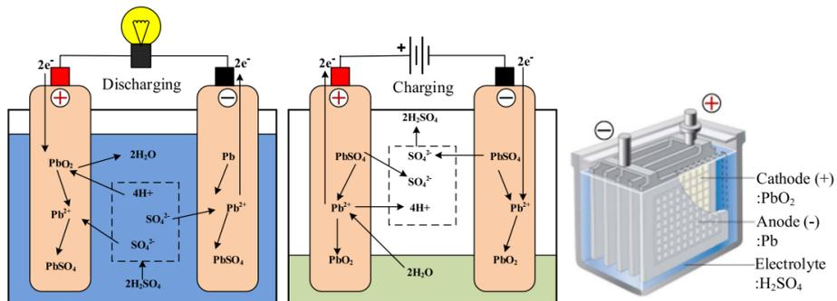
Figure 2.10 : Lead Acid batteries during charge and discharge[10].
