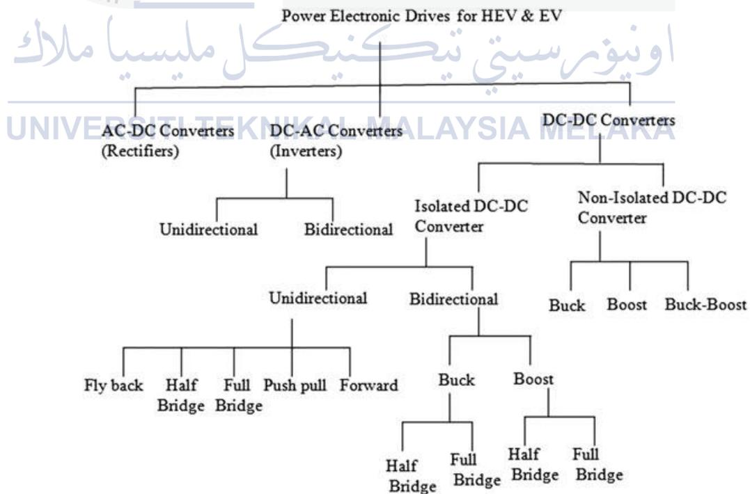
Figure 2.13 : Type of power Converter[3].
