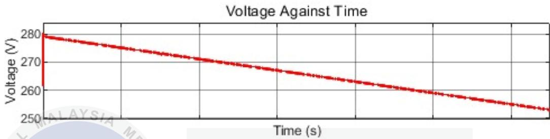
Figure 4.2 : Supercapacitor voltage for boost mode
