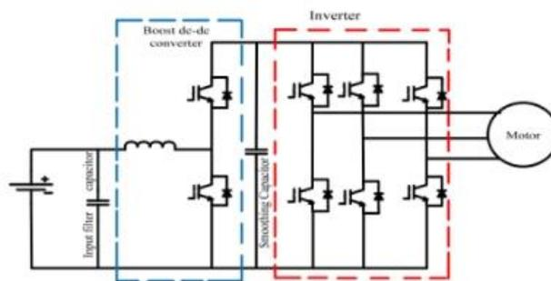
Figure 2.16 : Power control unit for hybrid electric vehicle[3]
