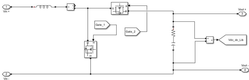
Figure 3.6 : Bidirectional DC-DC Converter
