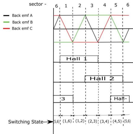
Figure 3.13 : Waveform of the back emf and Hall output
