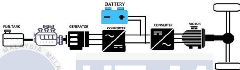
Figure 2.1 : Series drive train structure[3].
