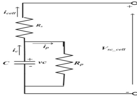
Figure 3.3 : Supercapacitor model
