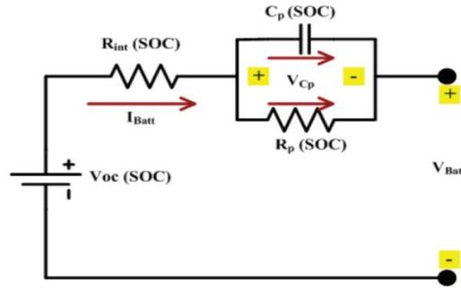
Figure 3.2 : Battery Model
