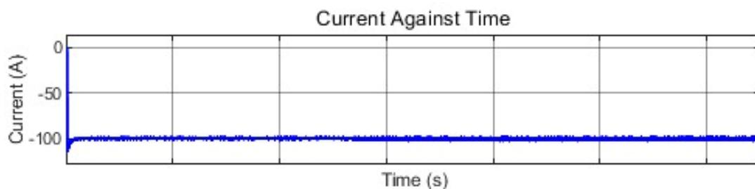
Figure 4.10 : Supercapacitor current for buck mode
