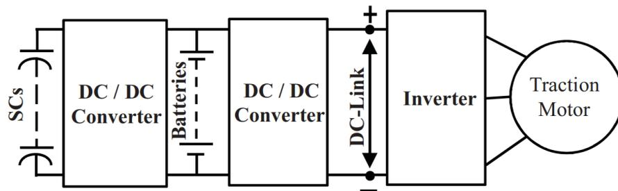
Figure 2.4 : Series SC/Battery Full Active[6].
