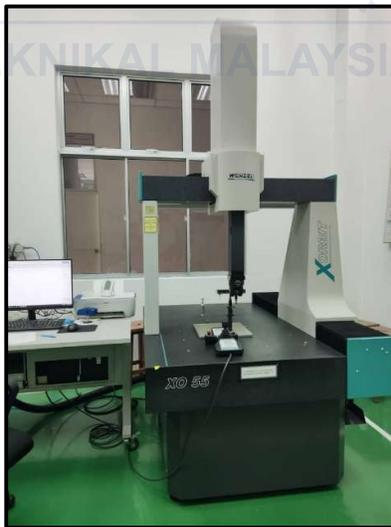
Figure 3.3: Coordinate Measuring Machine
