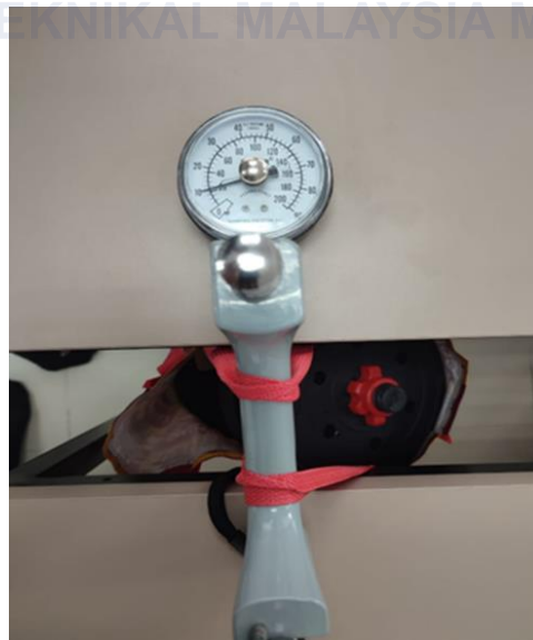
Figure 3.3: Calibrate a Jamar dynamometer with 10 kg dumbbells.
