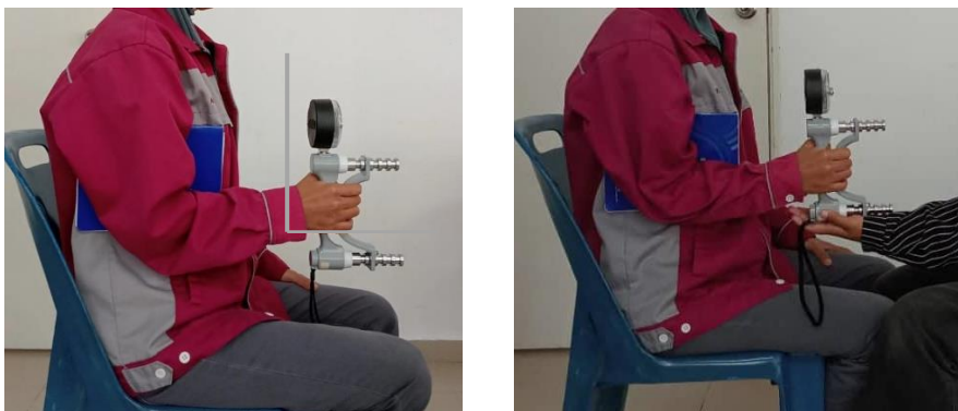
Figure 2.11: Left AHST (90-degree angle of elbow posture) and right SHAP (Support the weight of the hand dynamometer) protocol.
