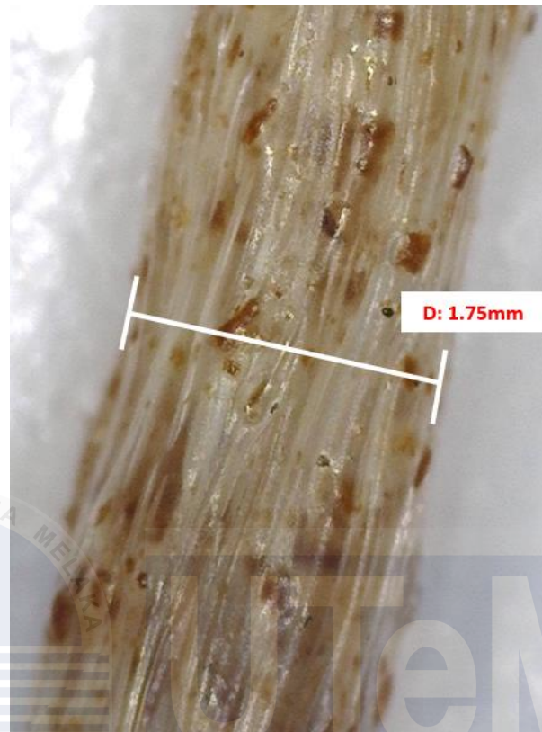
Figure 4.4: r-WoPPc filament dimension (mm)
