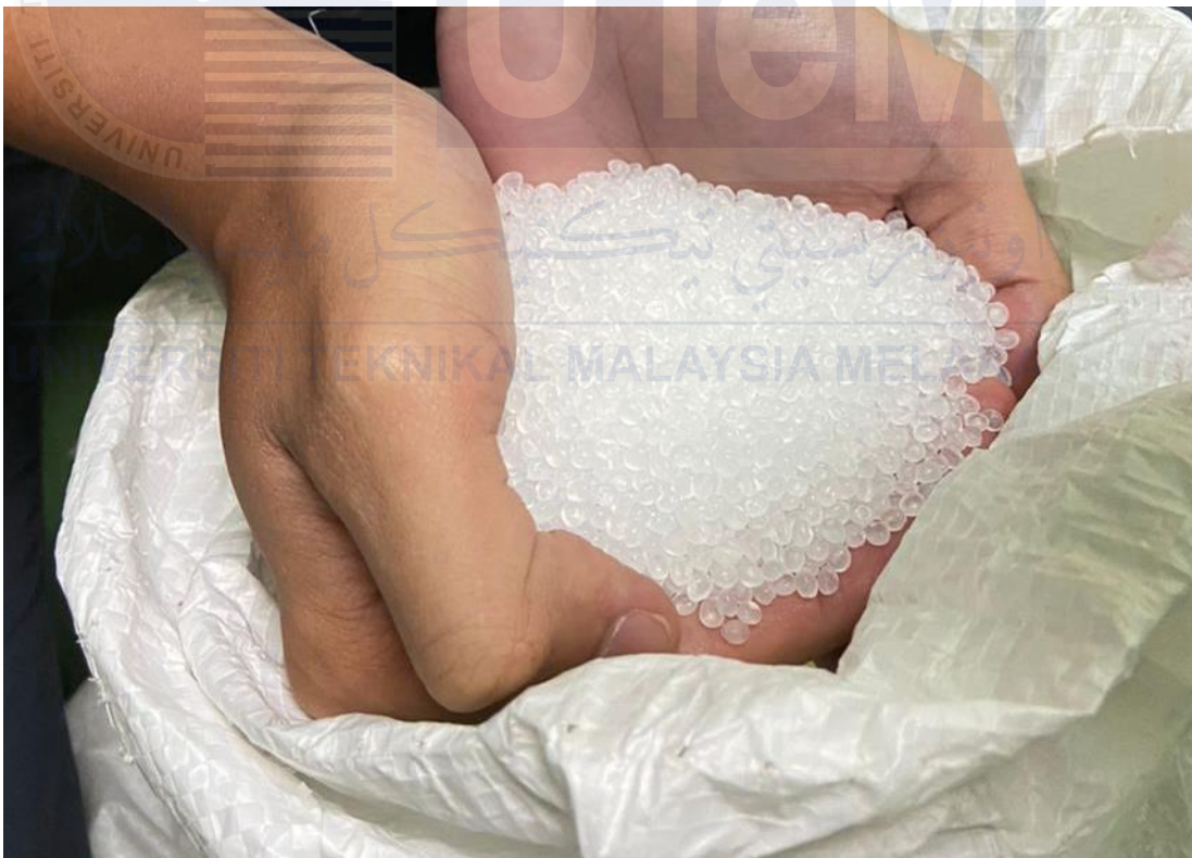
Figure 3.2: Granulated pellets of recycled PP
