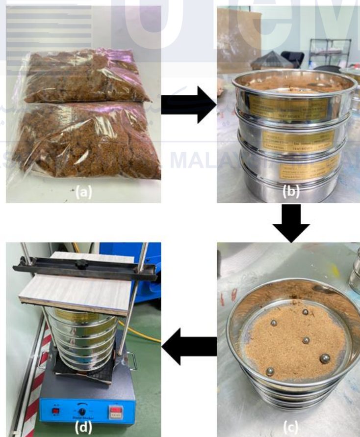
Figure 3.8: Sieve process; (a) clean wood fiber, (b) three different sieve sizes, (c) wood fiber is placed in sieve, (d) the machine is switch on for 30 minutes
