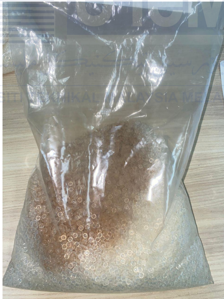
Figure 3.9 The mixed of wood dust and recycled polypropylene.
