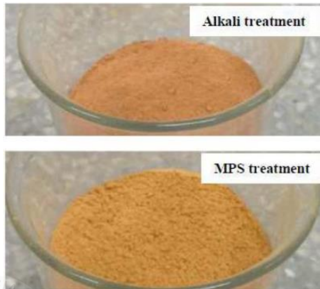
Figure 2.1 The Alkali and MPS treatment (Nattakarn Hongsriphan, 2016).
