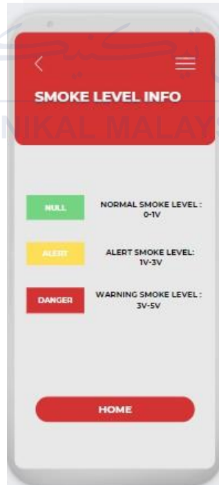
Figure 42: Smoke Level Info interface
